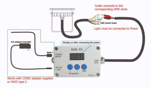
The coder is used for assigning an address to each light. Addresses can be changed or reassigned even after programming is complete if required.
