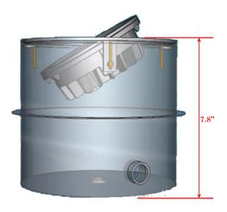
Fully adjustable SS niche which allows for an angle adjustment as well as 360° rotation of the light
